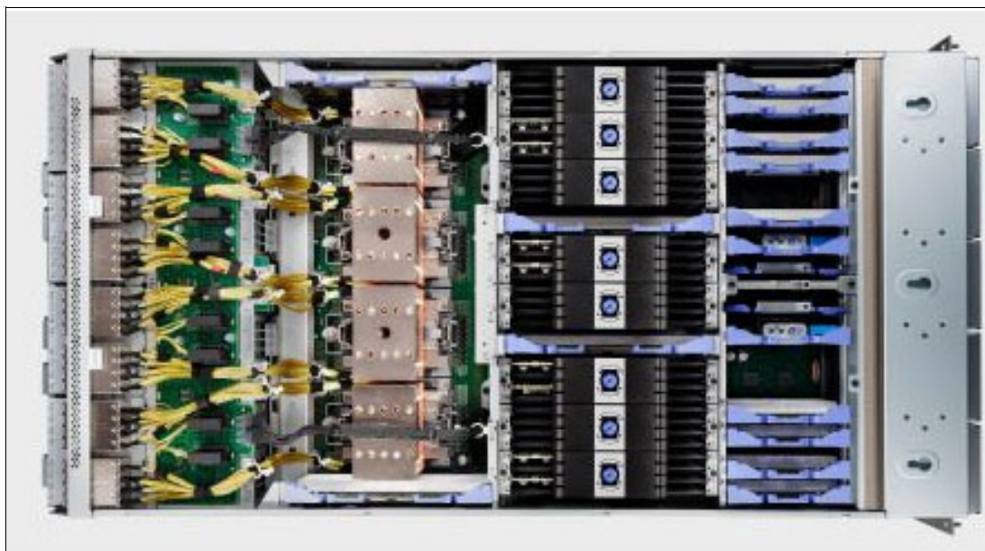
Figure 1-9 View of Power E1080 central electronic component drawer
