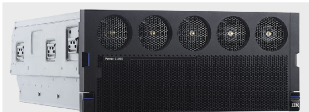
Figure 1-9 View of Power E1080 node
